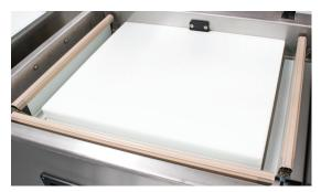
Three seal bars provide 64.5" of sealing bar length
